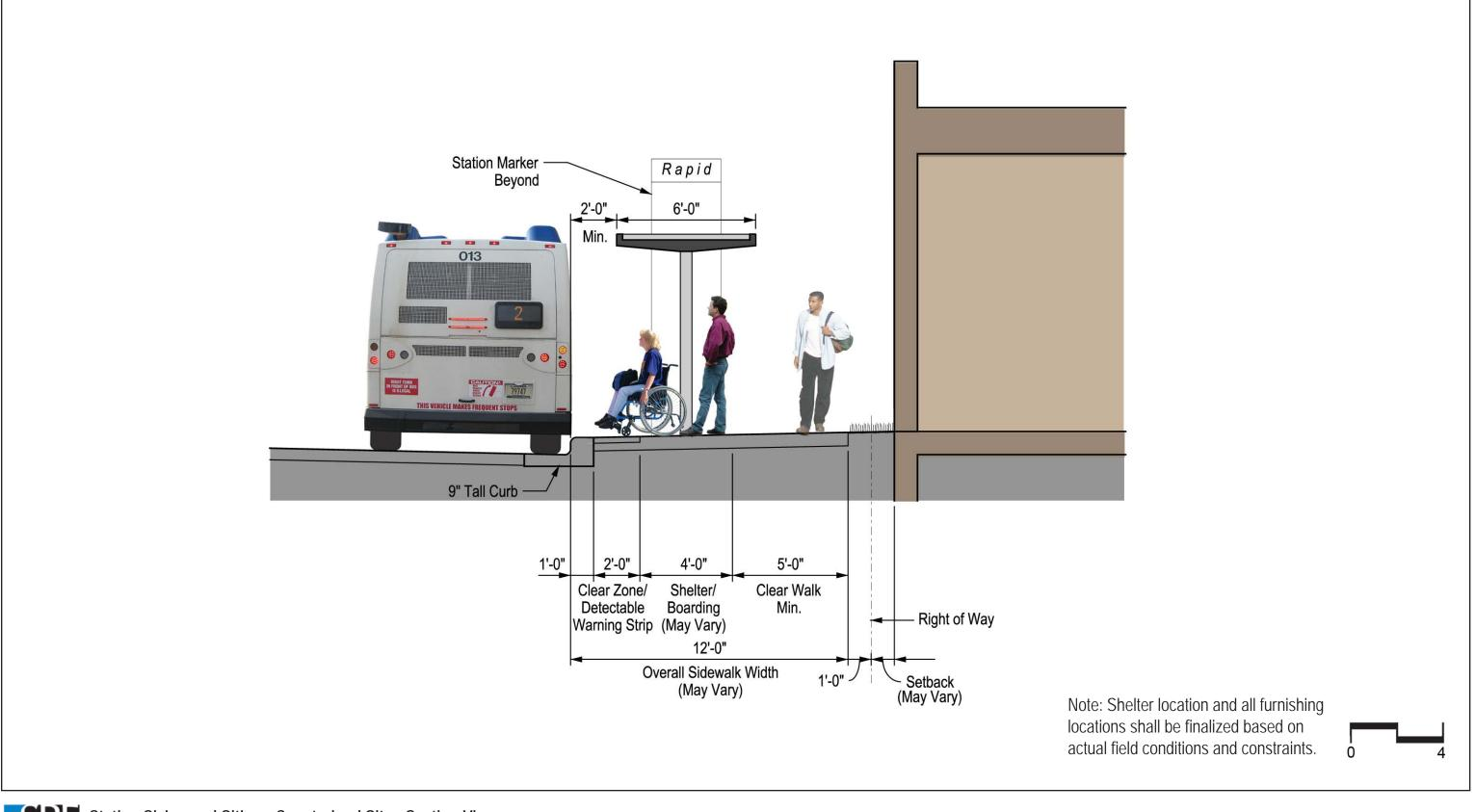
SRE Station Sizing and Siting - Constrained Site - Section View
