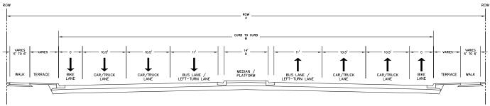
NOTE: PARK STREET REQUIRES WIDENING TO ACCOMMODATE THIS TYPICAL SECTION. MEDIAN NARROWED TO MINIMIZE CONSTRUCTION AND ROW IMPACTS
