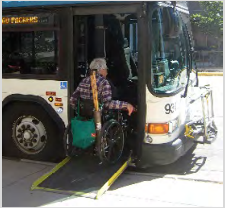
All Metro Buses are equipped with hydraulic ramps and wheel chair restraints.
